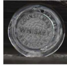
Seals. Made with small graphite molds.
